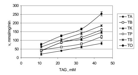
**Fig. 1.** The role of chain length of fatty acid in triacylglycerol (TAG) in lipolytic activity. The activity was determined by the standard titrimetric (continuous) method. Triacetin (TA) solution, mechanically stirred tributyrin (TB) emulsion and tricaprin (TC), tripalmitin (TP), tristearin (TS) and triolein (TO) emulsions prepared by ultrasonic treatment in 8% (w/w) gum-arabic aqueous solutions were used as substrates
