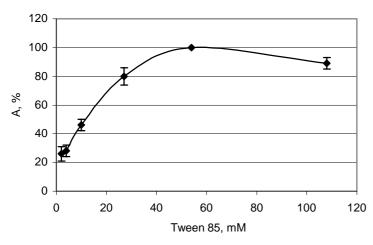
Fig. 3. Effect of Tween 85 concentration on lipolytic activity of *PmL*. The activity was determined by the standard titrimetric method in the presence of 2–108 mM Tweens concentration. 100% activity corresponds to  $144 \pm 4 \text{ mmol/mg} \cdot \text{min}$
